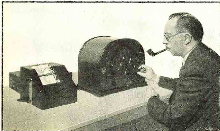
Figure 2. John V. L. Hogan tuning in a standard receiver to which is attached the simplified facsimile printer which can be used for home reproduction of illustrated news in "galley" form (news printed on a long length of paper tape)
